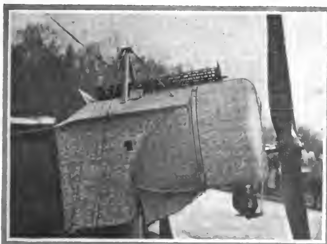
Engine housing and machine gun of a captured Fokker monoplane. The engine is a rotary Oberursel
